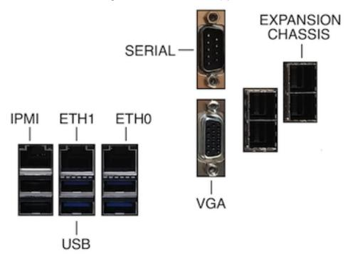
The connectors on the back of your EVO may be arranged differently, but the ports should be physically and functionally the same. The USB ports may be used to connect a UPS battery backup and/or keyboard. The video output is not needed in normal operation, but may be helpful for troubleshooting or inital configuration. If present, the serial port is RS-232 using 8n1, 57600 baud, Xon/Xoff. EVO typically has two built-in Ethernet ports, numbered as shown. In addition
